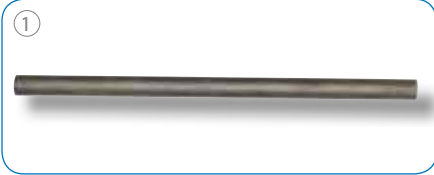
Blank cropped to size from C50 hardened and tempered steel.
