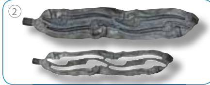
Hot forged in the double forging die. The excess burr is removed under an eccentric press
