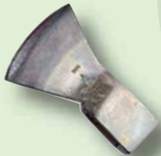
⑤ Permanent marking by means of a stamp bearing the manufacturer's symbol. Tempering (hardening and tempering) the cutting edge ensures hardness and toughness.
