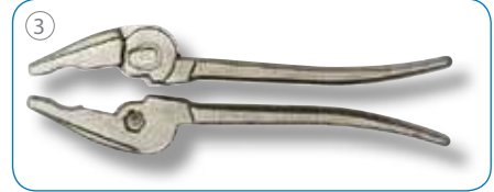
The blanks are "normalised" to obtain an even finer-grain, more uniform structure with optimum strength. After descaling, the blanks are calibrated for the following work steps.
