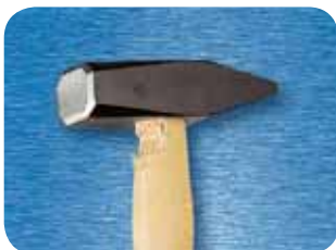
Unprotected hammer handle - After 30 impacts: Noticeable damage to the handle - risk of breakage!
