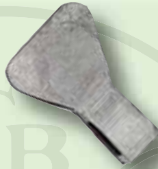
③ The glowing blade is beaten out on the forging roll.
